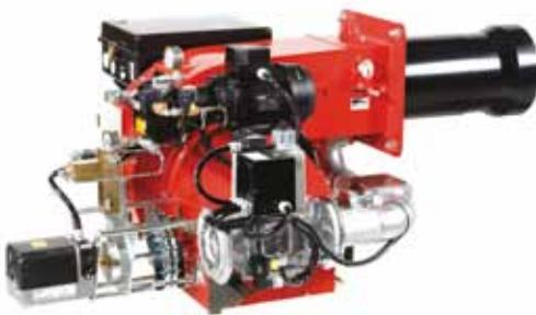
Dual fuel burners for gas and light oil at 2 stages progressive (hi-low flame) or PID fully modulating if optional modulation kit (digital type) and feeder (of temperature or pressure) are added.
