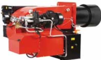
Burners for heavy oil two stages progressive or PID fully modulating. Equipped with Lamtec Etamatic OEM electronic camme. Fan at high pressurisation, combustion head with adjustment at high efficiency and high flame stability complete of servomotor for the opening of the air shutters, suitable for heavy oil up to 20°C to 50°C and for BTZ heavy oil.
