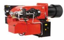
Burners for heavy oil two stages progressive or PID fully modulating with the addition of the optional system modulation kit plus feeder. Fan at high pressurisation, combustion head with adjustment at high efficiency and high flame stability complete of servomotor for the opening of the air shutters, suitable for heavy oil up to 20°E to 50°C and for BTZ heavy oil. Disposition rationalized of the components with accessibility facilitated for the operations of setting and maintenance.
