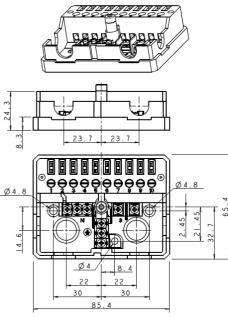
Socket NE Fig.3 Regarding the connection of the control units, provisions such as strain reliefs, sufficient earth terminals and neutral terminals should be present in the appliance or in external connection boxes.
