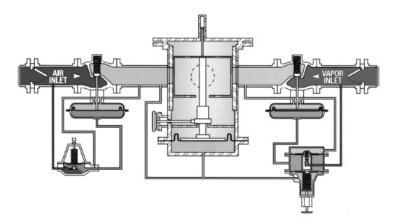
The air regulator also delivers control pressure to the diaphragm-actuated piston and controls the gas governor through a common sensing line. Consequently, regulated air pressure, regulated LPG vapor pressure and mixed LPG/Air pressure remain constant.
