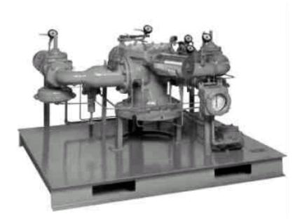
The **BLENDAIRE FVO** is designed to accurately mix LPG vapor with air over a wide range of ratios and deliver the mixed gas at a fixed designated pressure from 10 to 150 psi (0.70 - 10.55 kg/cm2). The Blendaire FVO's floating variable orifice valve make it specifically suited for high mixing accuracy and high discharge pressures without relying on instruments that are susceptible to calibration errors, electrical noise, or program faults.
